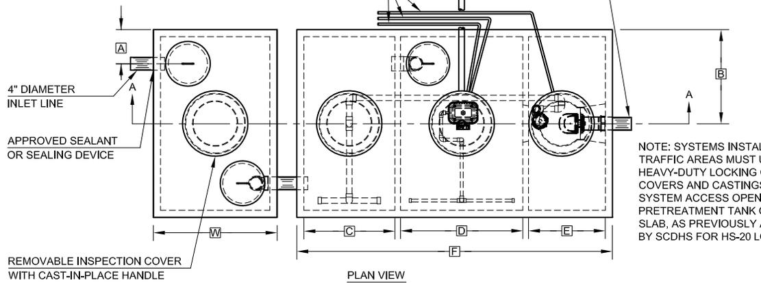
NOTE: SYSTEMS INSTALLED IN TRAFFIC AREAS MUST UTILIZE HEAVY-DUTY LOCKING CAST IRON COVERS AND CASTINGS FOR ALL SYSTEM ACCESS OPENINGS AND PRETREATMENT TANK COVER SLAB, AS PREVIOUSLY APPROVED BY SCDHS FOR HS-20 LOADING.
